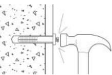
the proper embedment. This anchor is not recommended for use overhead.
